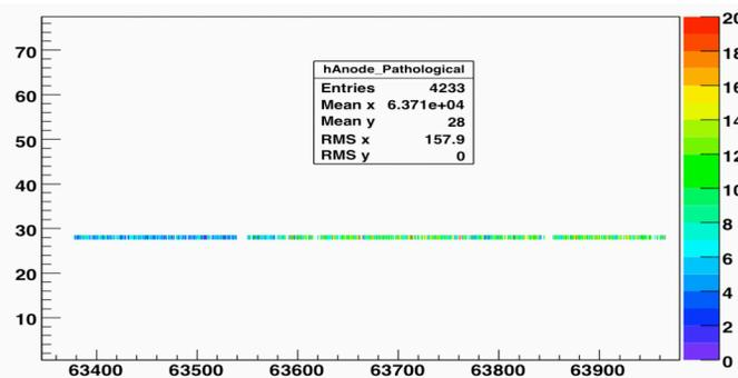
The pixels which show the EVH & ! EH Pathology seem to be associated with the same anode, #28. Conclusion, probably due to a faulty EVH threshold discriminator.
