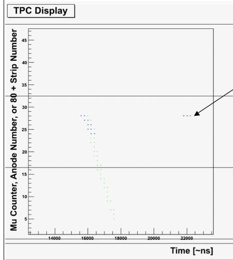
Close up of an event with 3 EVH Pixels, the last of which has no corresponding EH.
